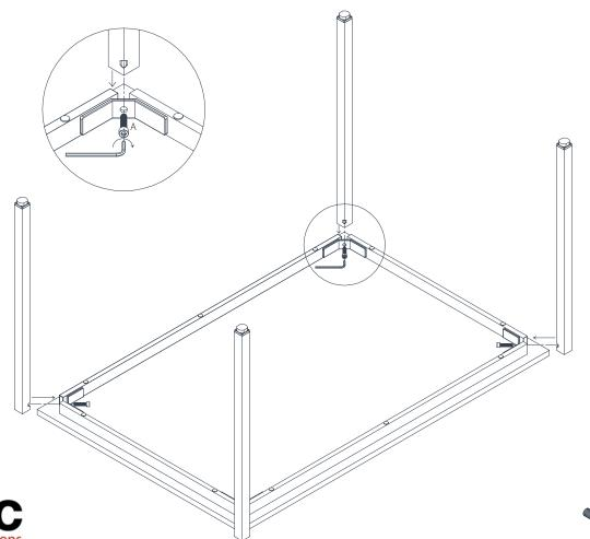
NOTE: Ensure arrow is facing direction of the screw head before tightening
