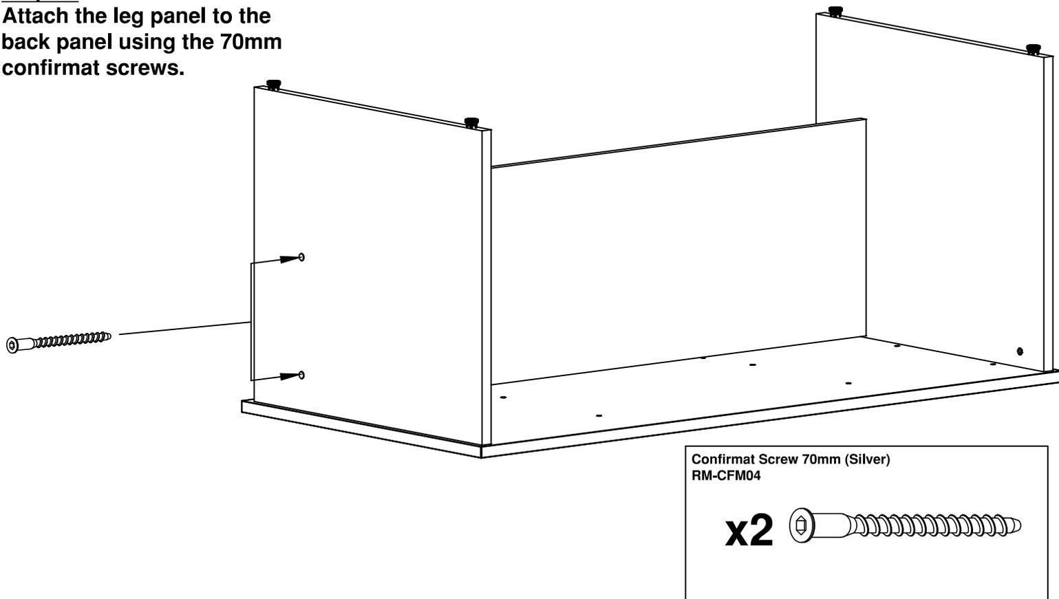
Matching adhesive caps are provided to cover any visible screw heads or cam fittings.
