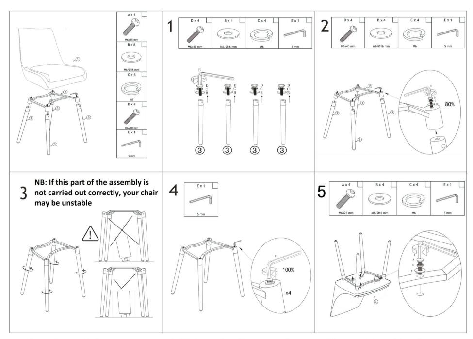
Notice: Please tighten screws up initially using fingers only to avoid cross threading the screws
