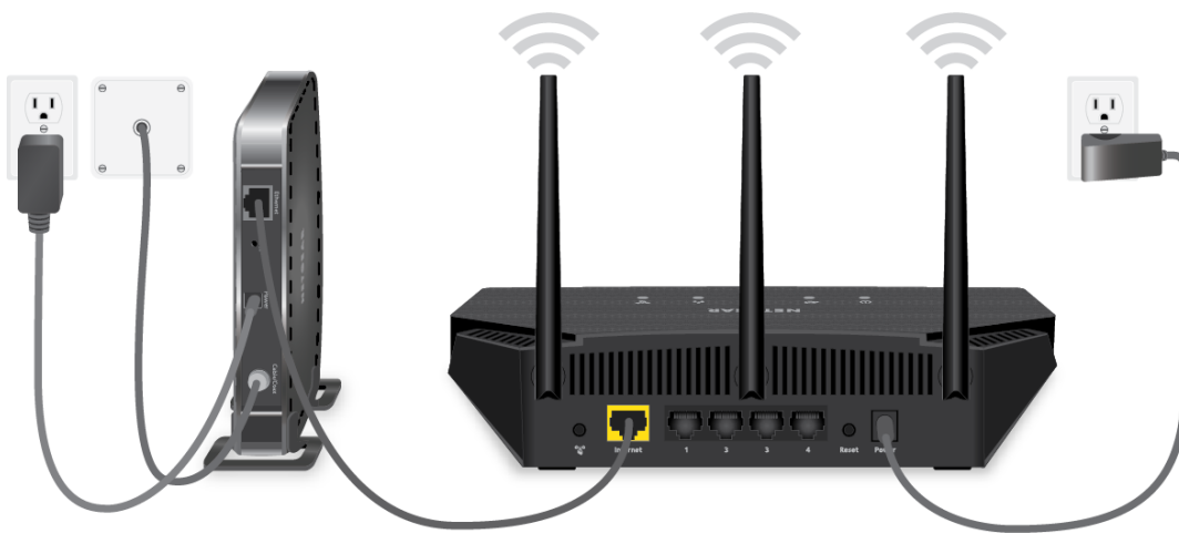
Figure 6. Cable your router
