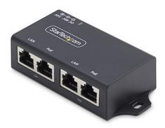
This 2-port multi-speed PoE+ injector serves as Power Sourcing Equipment (PSE) and enables Ethernet speeds of 10/100/1000Mbps. This mid-span inline injector can transmit network data and power up to 328ft (100m) for two Powered Devices (PD).
