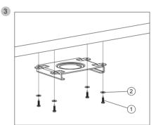
Install the mounting panel with four screws 1 and four washers 2.
