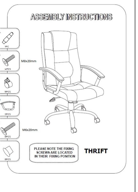
Please note the fixing screws are located in their fixing points . Do not tighten bolts fully until you have completed assembly.
