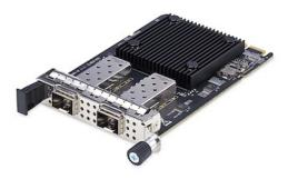
The 2-port 10Gbps OCP network interface card with the Intel X710-BM2 controller adds two open SFP+ slots to a server, increasing connectivity options and network performance.
